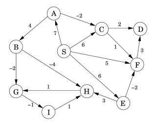
Draw a table displaying the intermediate values h (the distance estimates for the nodes), and draw the final shortest-path tree.
